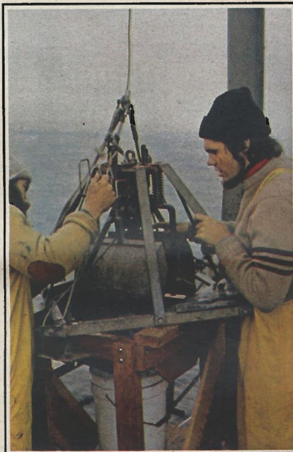
Scientists Mark Silverstein and Dave Wilson ready the spring-loaded grab for a trip to the ocean floor to collect sea life.
