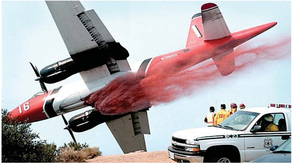
This P2-V is a converted US Navy submarine chaser, now assigned to fighting fires throughout North America. This plane, or one like it, flew over the author's farm to slow the wild fire's advance. Photo by Leo Jarzomb, San Gabriel Valley Newspaper Group.
